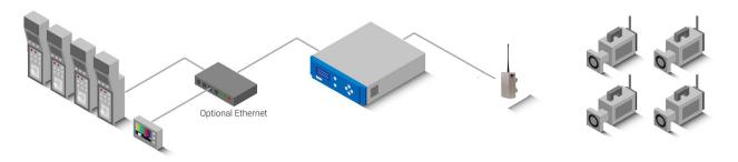
Cascade (Mix multiple manufacturers on a single frequency)
